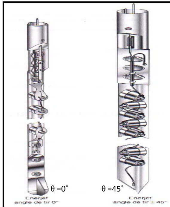
Figure II.6 : EXEMPLES DE SUPPORTS SANS PROTECTION EXTÉRIEURE.
