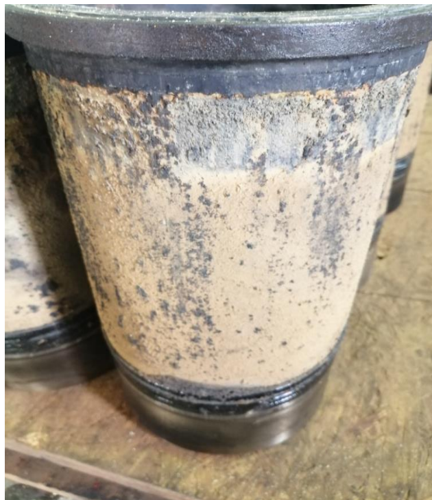
Figure 17 (III.3). Chemise corrodé
