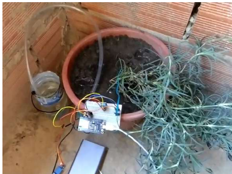
Figure 4.7: Pump part of the irrigation system prototype
