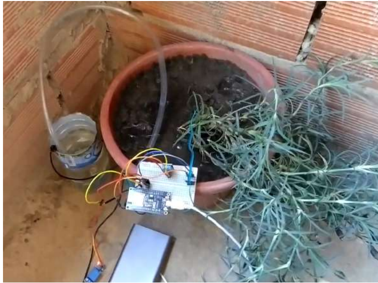
Figure 4.8: Pump part of the irrigation system prototype
