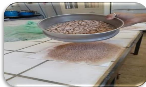
Photo3: tamisage (tamis 100 \mu\text{m} )
