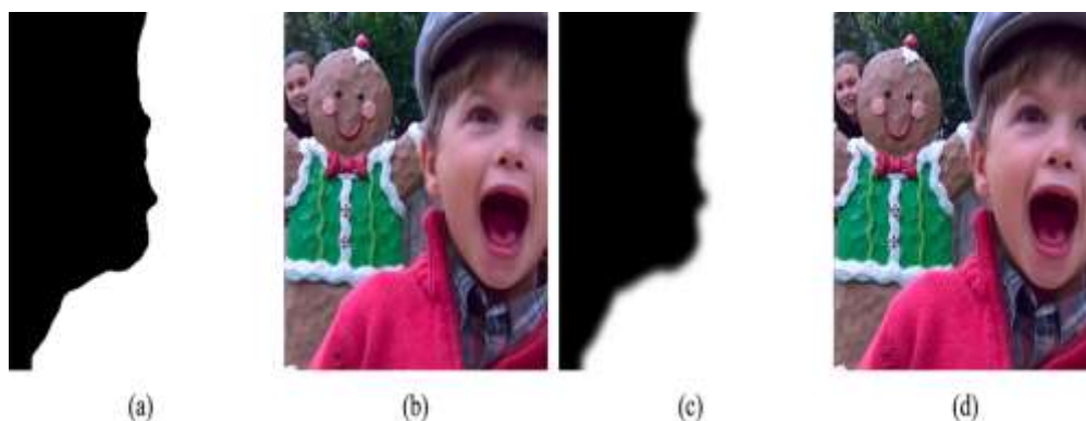
Fig (II.11): Consistency verification and fusion (a) Initial decision map (b) Initial fused image (c) final decision map (d) fused image.
