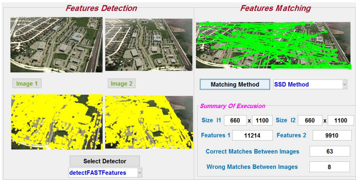
Figure1II.20: Detect FAST features and SSD matching method
