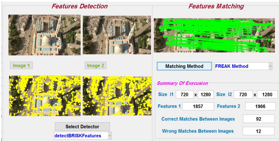
Figure 1II.19: Detect BRISK features and FREAK matching method
