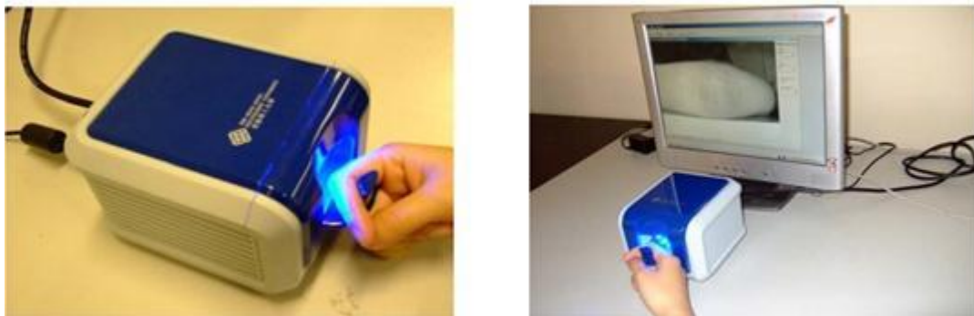
Figure III.2 : Appareil d'acquisition d'image FKP.
