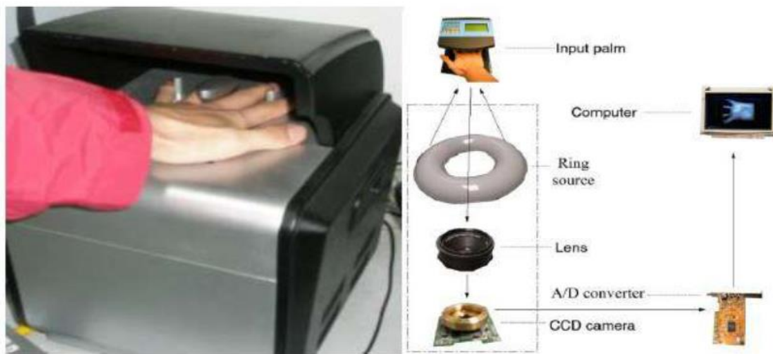
Figure III-3 the structure of the palmprint image acquisition device.
