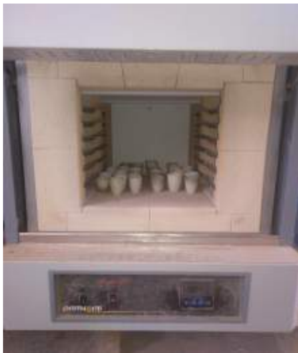
Photo5. The silica crucibles into the muffle furnace at 360°C
