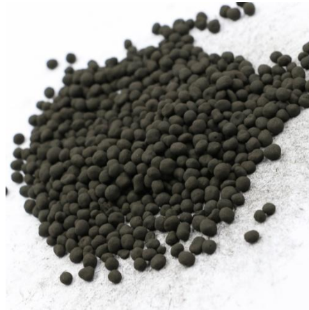
Figure III-16. Bead Activated Carbon (BAC) activated carbon.
