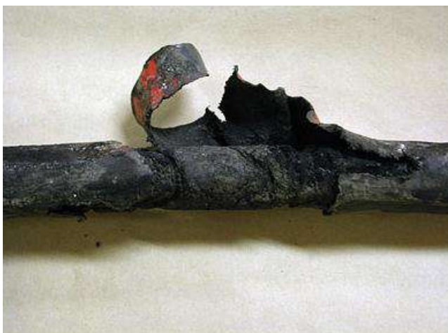
FigureI.24. Cable failing from the outside in [18]
