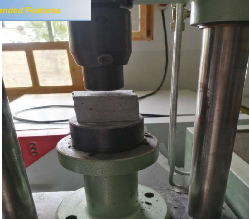
Figure21: Essai de compression
