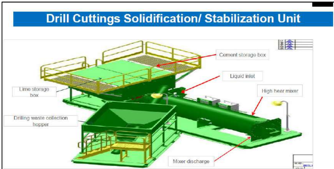
Figure III-6- Unite de soldification[27].
