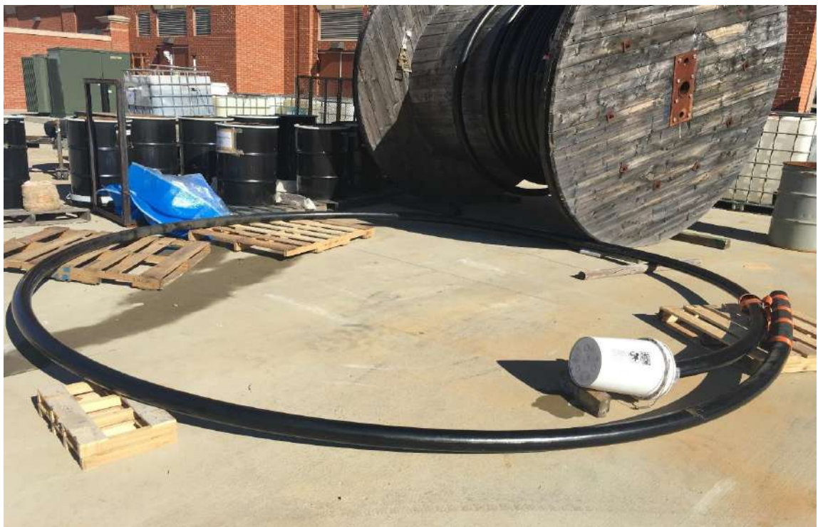
FigureIII.1: XLPE Cable Sample The cable sample shown in Figure 5 is 138 kV XLPE power cable with copper conductor. [5]
