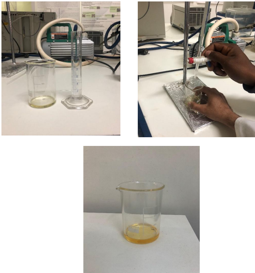
Figure 15: Experimental setup of the Acid Number.
