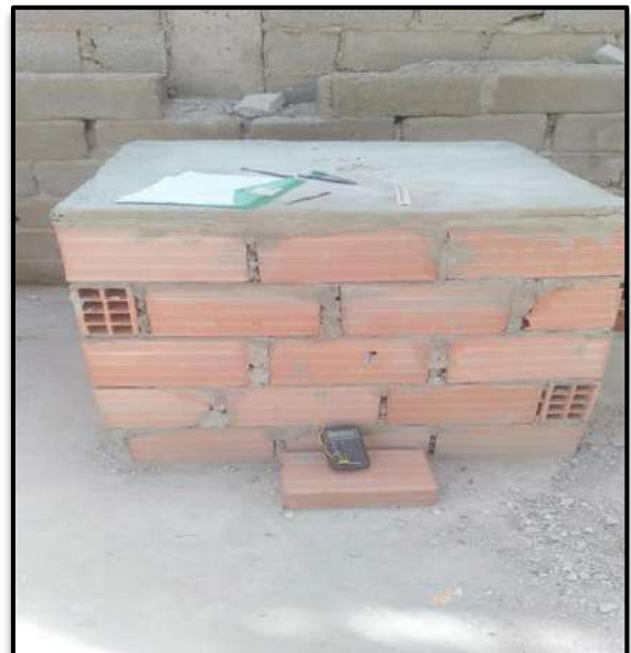
Figure III.14 Dalle en béton armée P1
