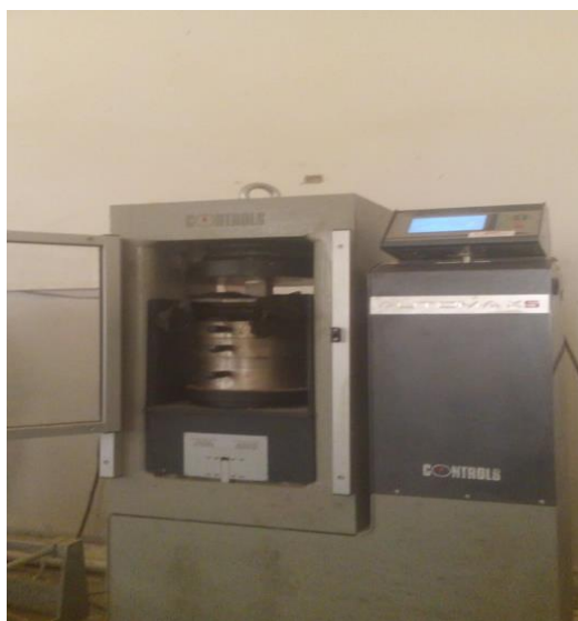
Figure II.1 : Essai de compression
