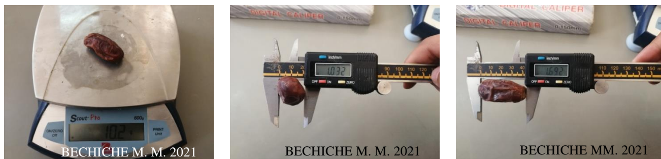
A. Weight measuring B. High dimension measuring C. Lenth measuring
