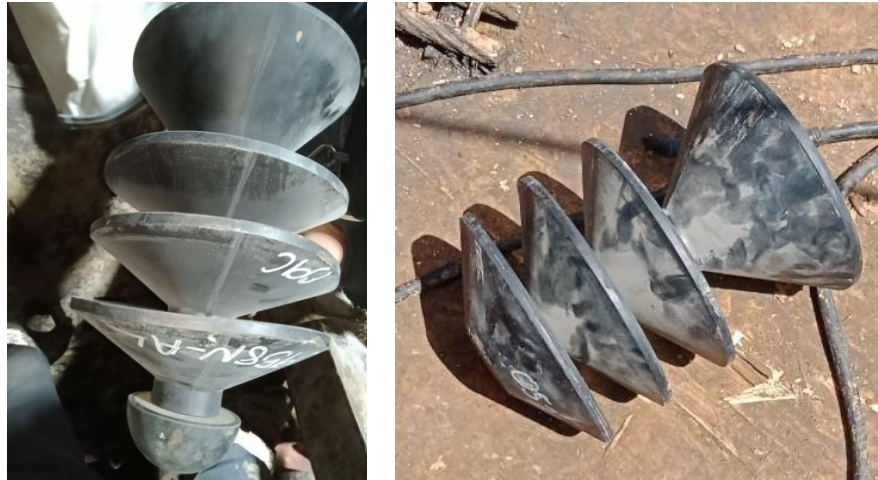
Figure.III.3 : Bouchonne de cimentation. [02]
