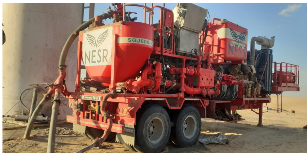
Figure.III.6 : Unités de cimentation. [02]
