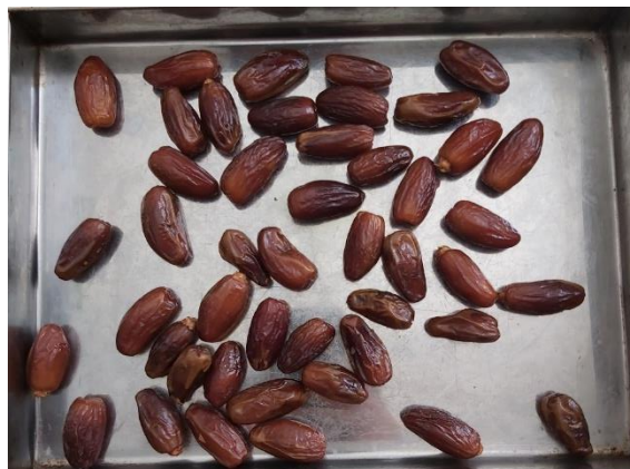
Figure IV. 9: photo des dattes après séchage a condition ( T = 70^{\circ}\text{C} , Q_v = 18 \text{ m}^3/\text{h} )
