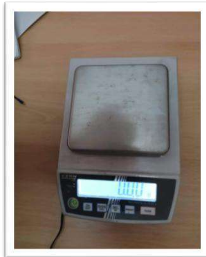
Figure III. 6: Balance KERN ABT 220-4M 200g/0.1g
