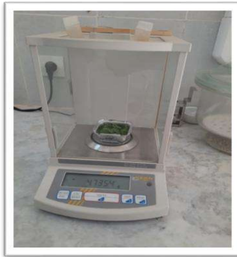
Figure III 9: Balance KERN ABT 220-4M 200g/0.1g.
