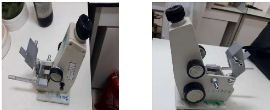
Figure 10 : ABBE refractometer for the determination of the refractive index.
