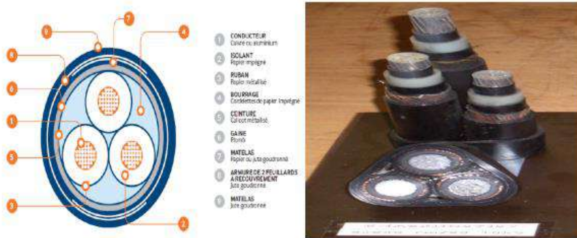
Figure I.12. Composition of a three-pole cable [11].
