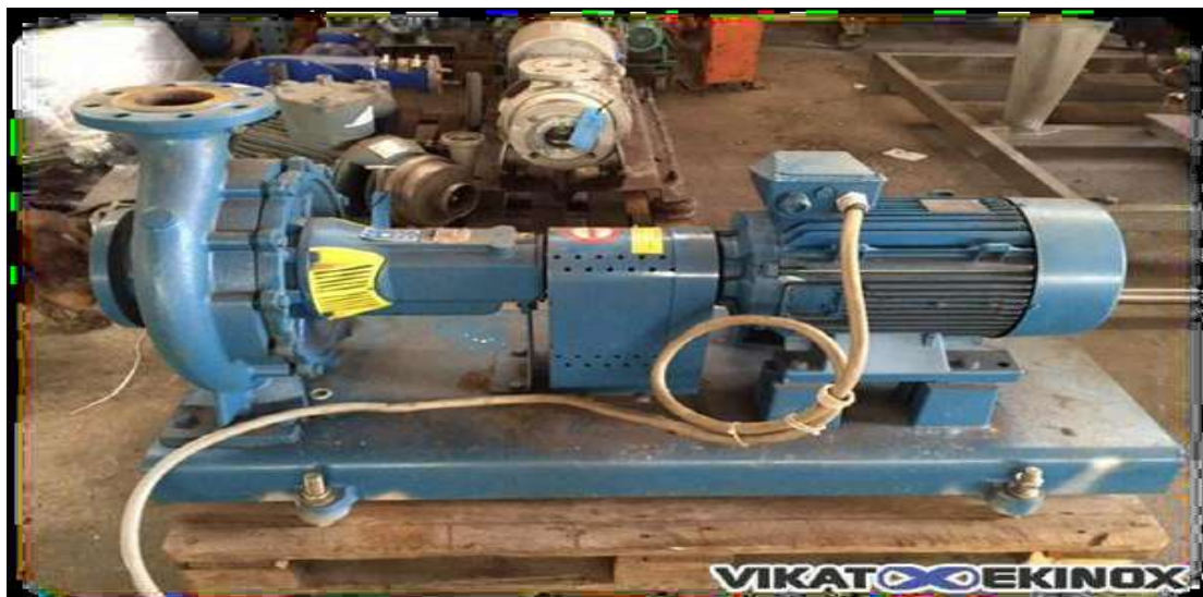
Figure (II-4)-Pompe centrifuge
