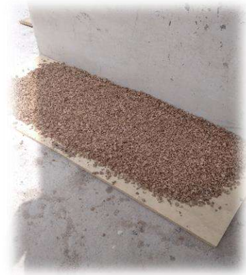
Photo II.5: Sechage de gravier
