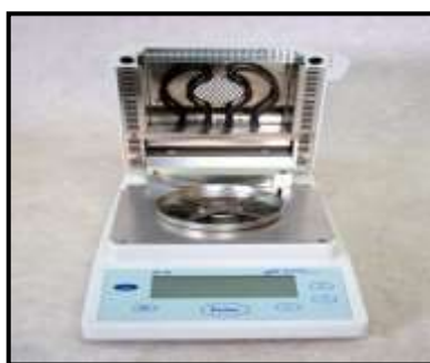
Figure II. 3: Humidity Analyzer IR35 Denver Instrument for initial moisture measurement.
