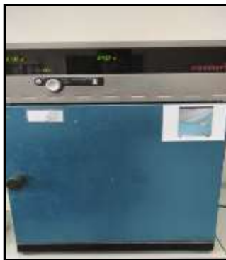
Figure II. 2: Programmed temperature drying oven (type: MEMMERT UFB 400 UNIVERSAL OVEN) for Total Solid Test.
