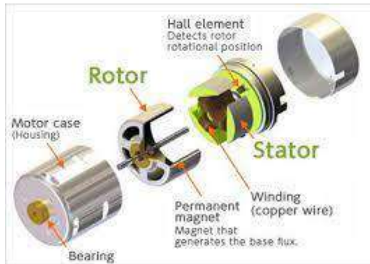
Figure (I .12)Construction de BLDC
