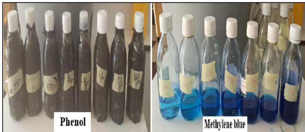
Image II-9: The various concentrations in order to create a calibration curve
