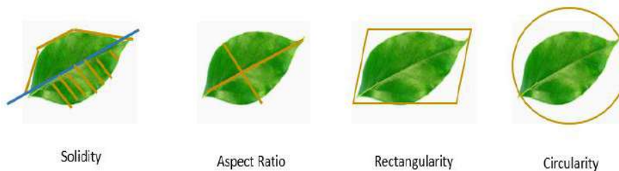
Figure 7.3: Morphological features. (a). solidity, (b). Aspect Ratio, (c). Rectangularity (d). Circularity.
