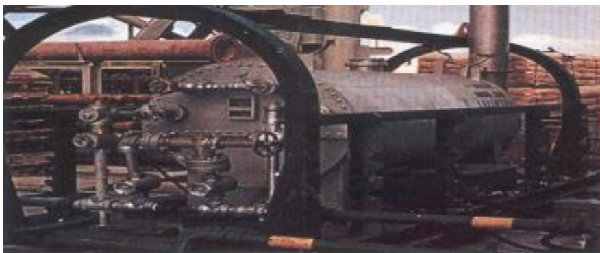
F.3.3- (Heat exchanger)
