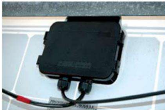
Figure 1.6. A junction box
