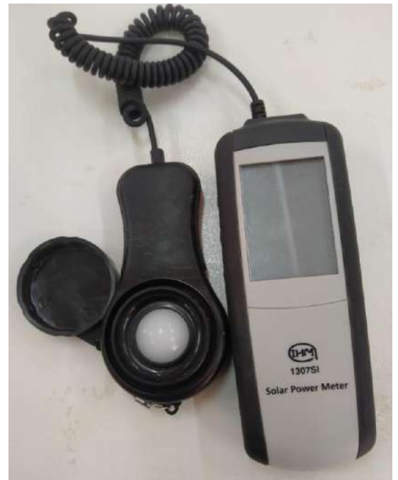
Figure IV.9: Solar Power Meter
