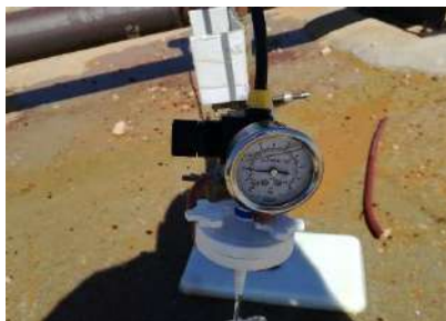
Figure II.1: Measure SDI of well
