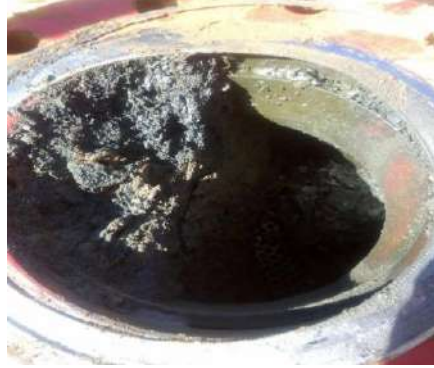
Figure III.100: Deposit inside ENMAX device.
