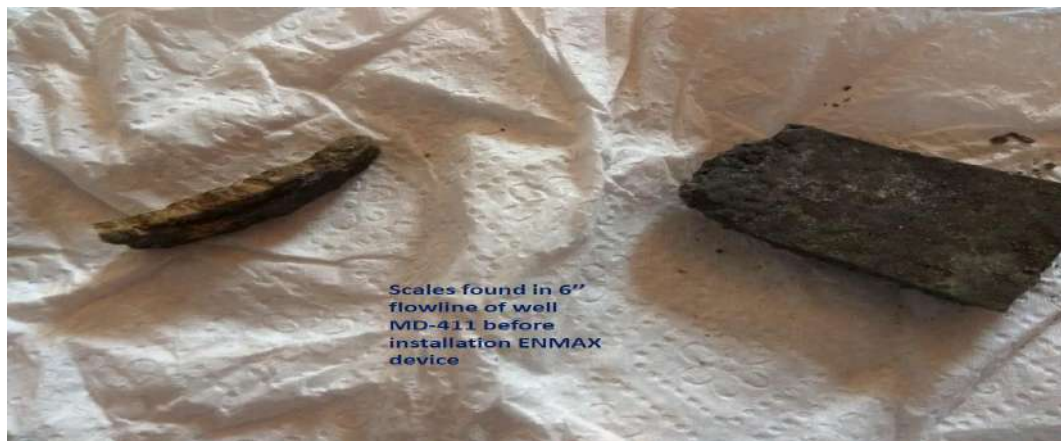
Figure III.82: Deposits formation on the flowline of well MD-411.
