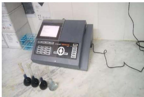
Figure II.10: Discoloration of the solution and Control of the anti-deposit concentration by the UV-Visible spectro-photometer
