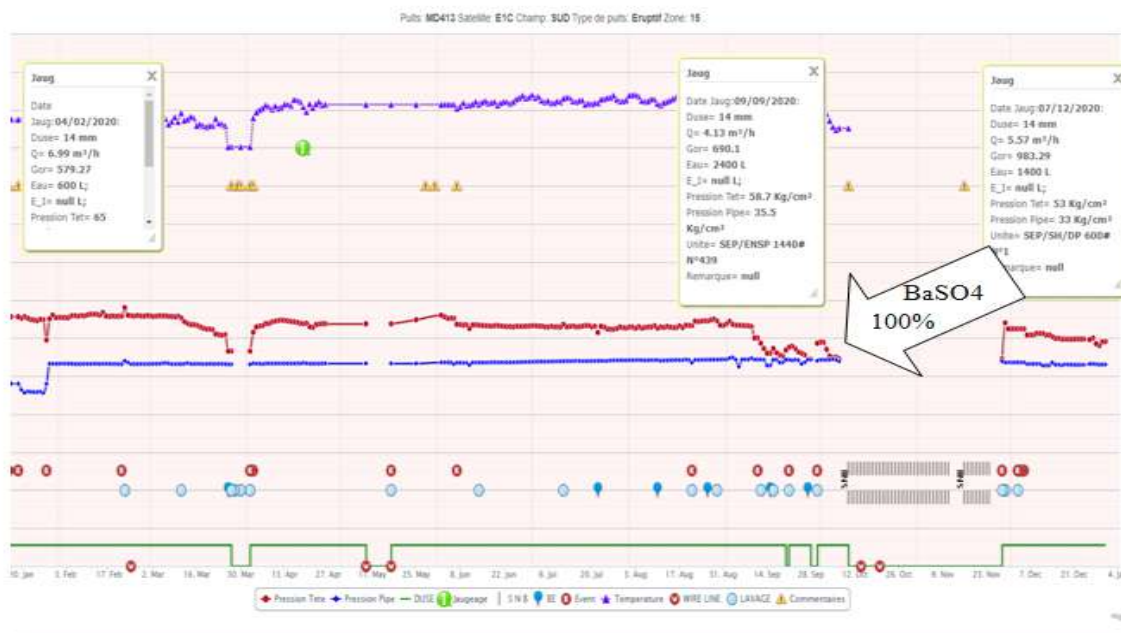
Figure III.71: MD413 Well production profile - After the use of CHIMEC 1264 Inhibitor. (DATA Bank, SH ,2020)
