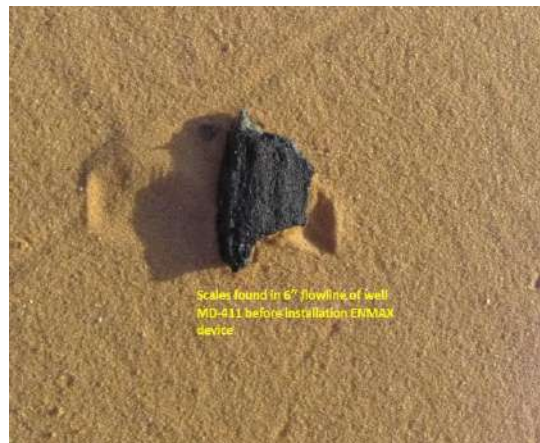
Figure III.97: Scales found in the flowline of well MD-411.
