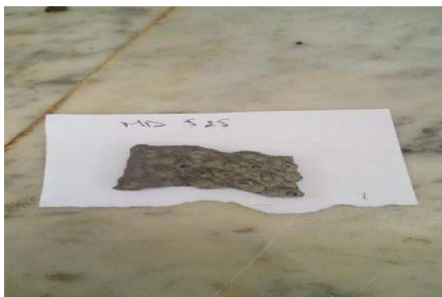
Figure III.39: MD 525 well deposit (Arbaoui, 2018).
