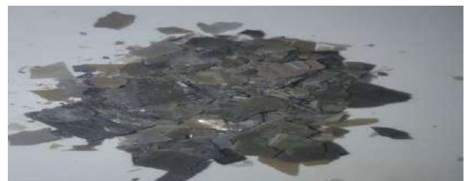
Deposits Inside Line 2'7/8, snubbing
