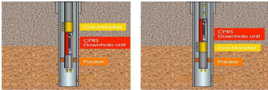
Figure I.53: CPRS Downhole unit (Enmax Technology (Shanghai) Co, 2012).
