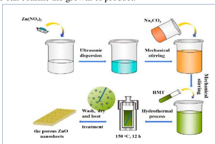
Figure I.11. Schematic Illustration of the Hydrothermal Synthesis of ZnO nanosheets. Reproduced from MDPI [278].
