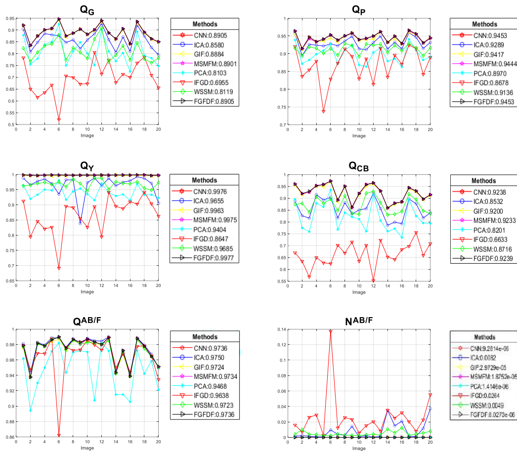
Figure 5-10 The performance of different multi focus fusion methods on a dataset of 20 grayscale images.
