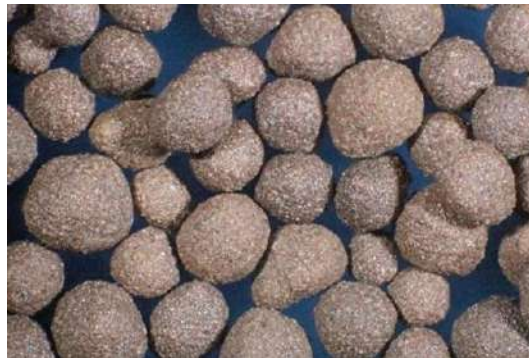
Figure I-7 Agents de soutènement ISP (par Saint Gobain) (Assem, A.I, al, 2017)
