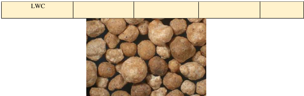
Figure I-9 Agents de soutènement LWC (par Carbo Ceramics Inc.)
