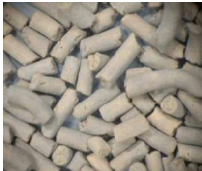
Figure I-13 Agents de soutènement Rod-Shaped (McDaniel et al., 2010).
