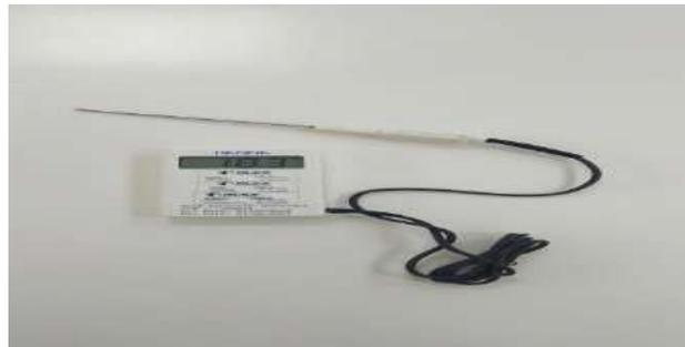
**Figure II-5:** Thermocouple [07]
