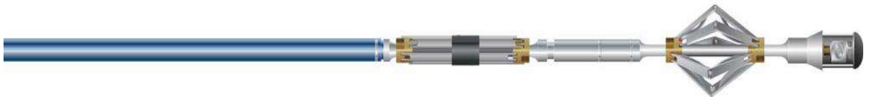
Figure II.12 : Le USIT (Ultra Sonic Imaging Tool)
