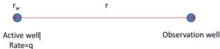
Figure II. 11 Active and observation wells, interference or pulse test (Earlougher, 1976).
