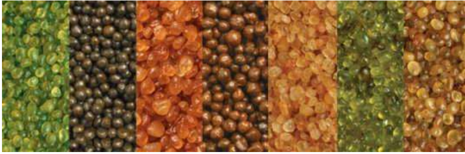
Figure II.7 DIFFERENTS AGENTS DE SOUTENEMENT (PROPPANTS) [23]
