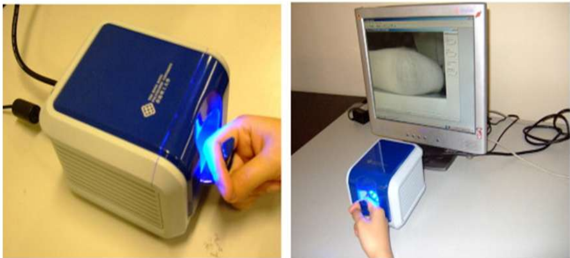
Figure 2.6 – The device used to collect finger knuckle print images.
