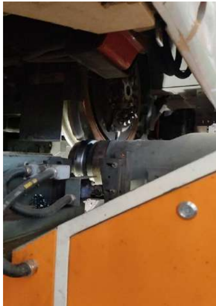
Figure 3- 28. The arm drive rollers contact on the wheels
