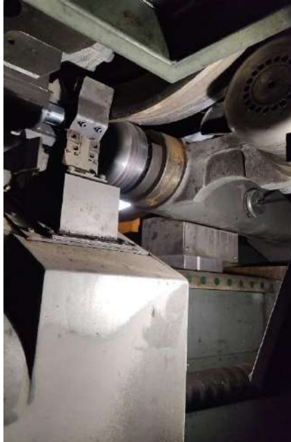
Figure 3- 26 : machine wheel trainer arm rolling the wheel
