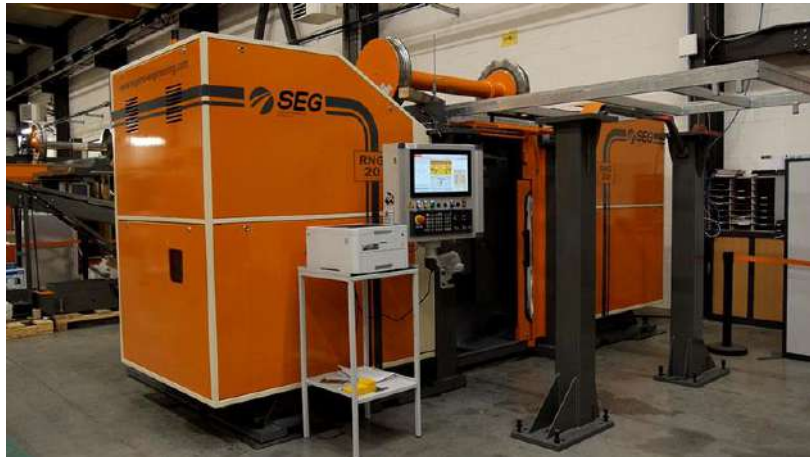
Figure 3- 4 Wheel Reprofilng Machine RNG 20 (not installed)[13]
