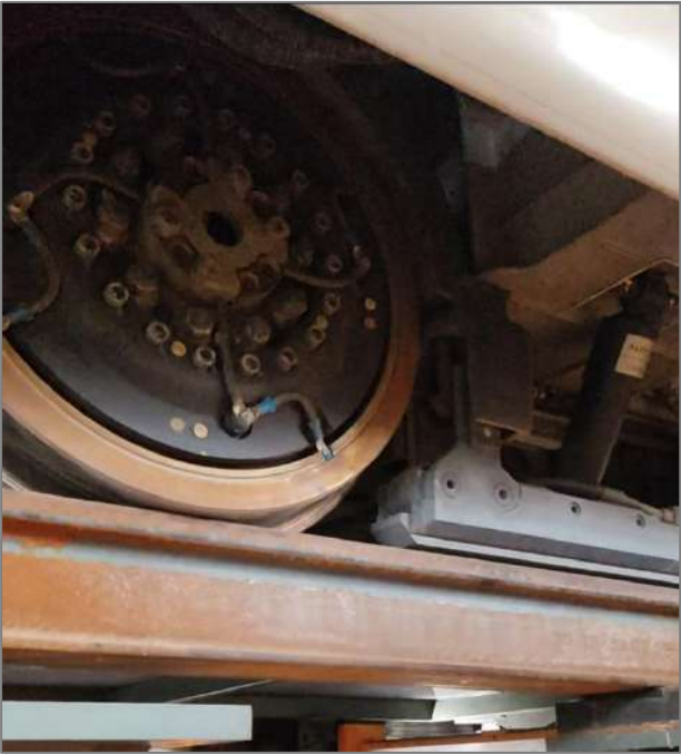
Figure 3- 2 Tram wheel on rail
