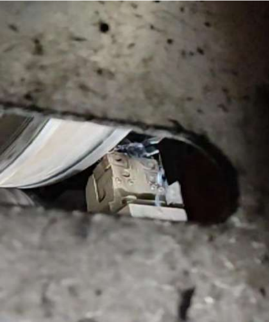
Figure 3- 30 : Reprofiling the wheel
