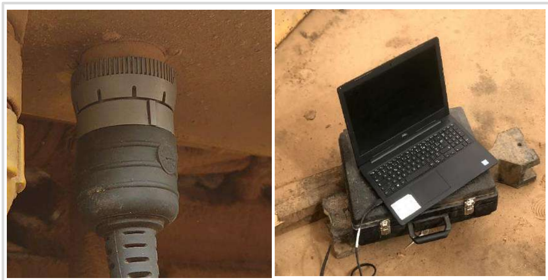
Figure 3- 10 : Generator connected to the PC via ET port
