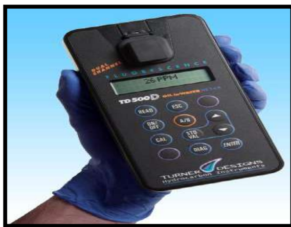
Figure IV.3: TD500 oil in water meter
