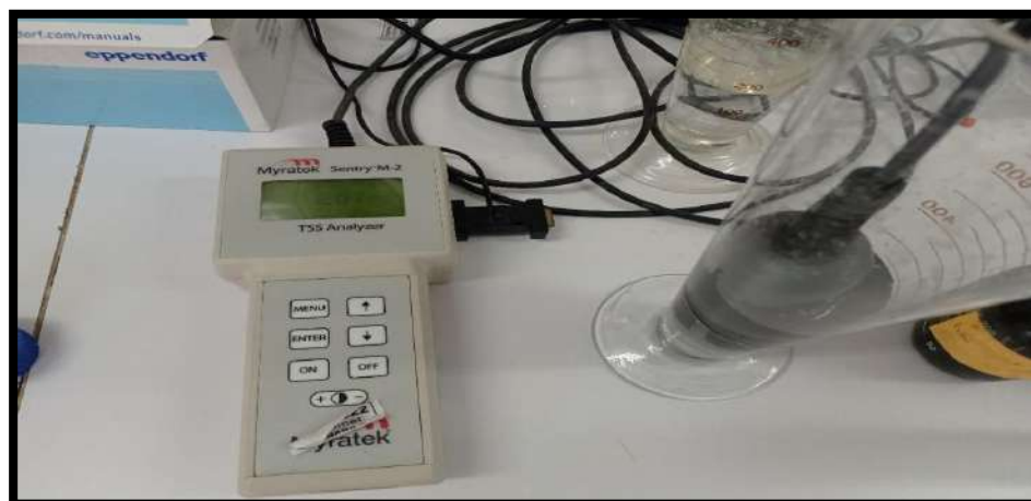
Figure IV.5: Suspended Matter measurement
