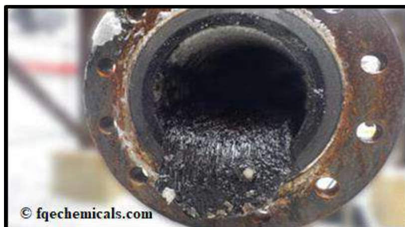
Figure (II.2): Asphalt deposition.
