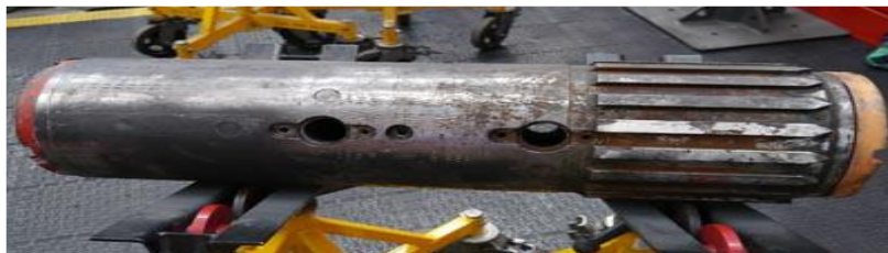
Figure II.3. Cutaway View of Upper Splined Kelly Guard.
