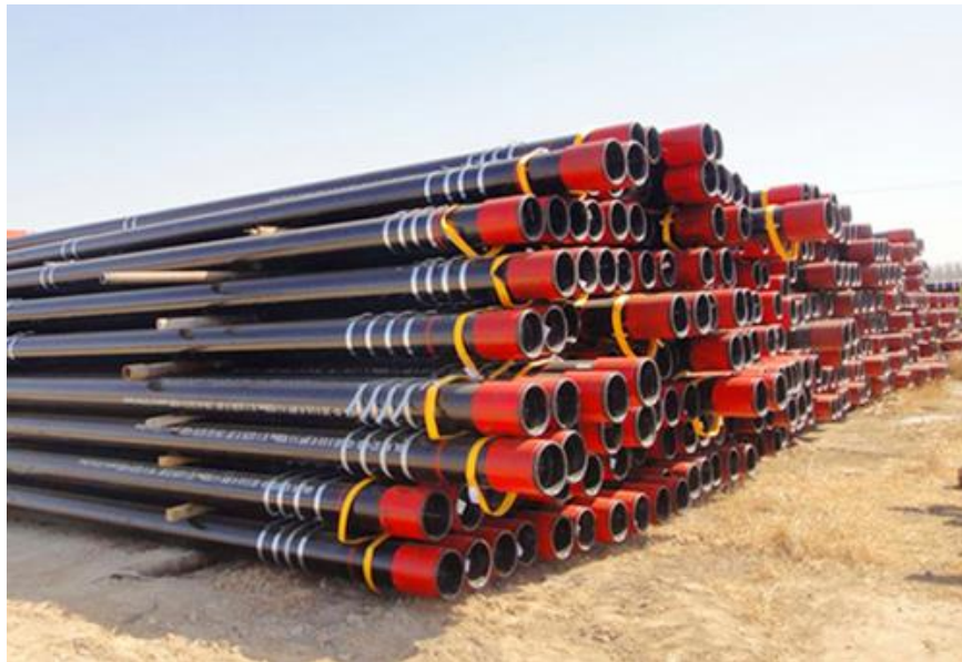
Figure II.8: Tubing de production
