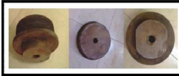
Figure(I.3): Image of fixed or positive wellhead chokes with 32/64 in or 1/2 in apertures [7].
