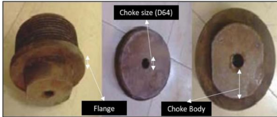
Figure(I.6): Image of fixed or positive wellhead chokes with 32/64 in or 1/2 in apertures.
