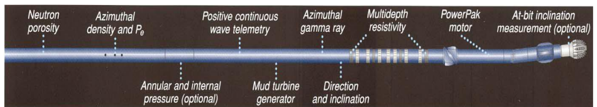
Figure I.13: Système LWD "Geo-steerable" [5]
