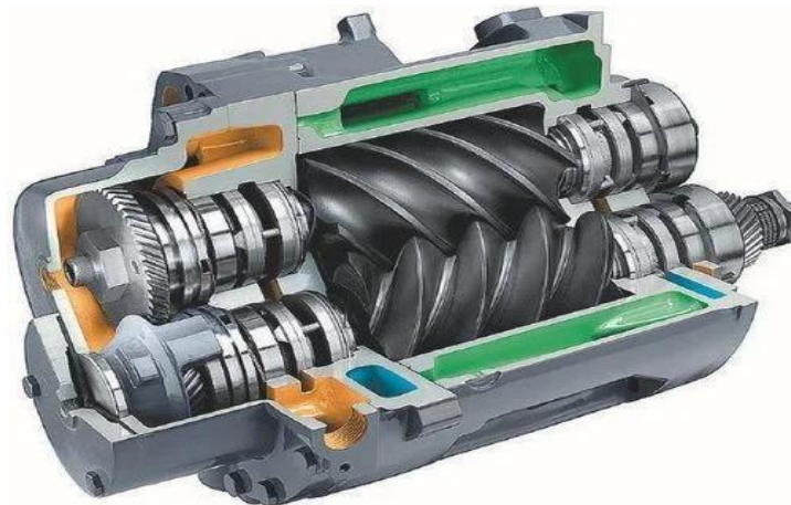
Figure I.5: Rotary screw compressor
