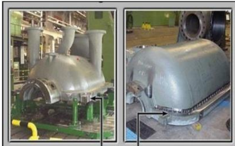
Figure I.13: Compressors with horizontally open bodies
